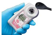
The PAL-10S is a digital hand-held compact refractometer that measures Urine Specific Gravity. To operate, simply place a drop of urine on the prism surface and press the START key. The Urine Specific Gravity value will be displayed on the LCD.
