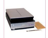
The microSCAN is an affordable low-cost gel documentation system for scanning colorimetric 1-D and 2-D protein gels, as well as blots and TLC plates.
