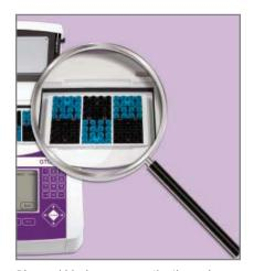
Blue and black squares on the thermal cycler block aid identification of each of the six 4x4-well temperature zones.
